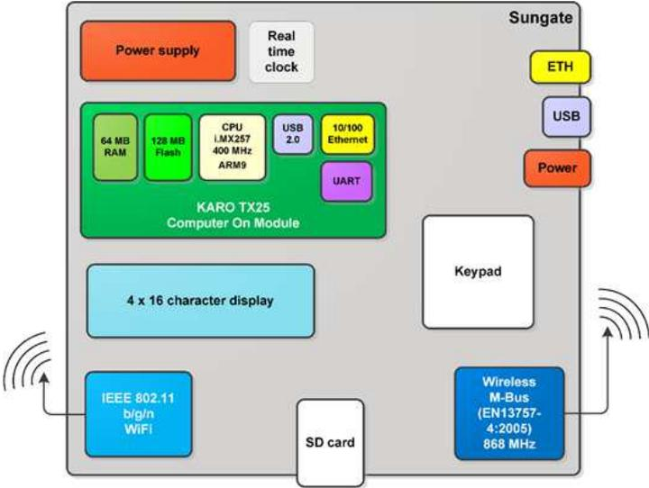
Letrika communication gateway differs from other micro inverters gateways in embedded Linux operating system, which allow virtual any software/drivers written for this operating system to be used on our gateway. Even more, software from gateway can be easily ported to Raspberry PI and other Linux based systems.
