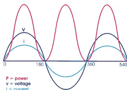
Current is in phase with grid voltage. This is typical diagram for resistive load.
