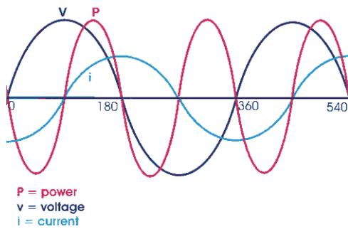
Purely inductive power. Current is lagging  $90^\circ$  behind the voltage. Power oscillates at twice of grid frequency. Average power in this case is 0, since there is no useful work possible.
