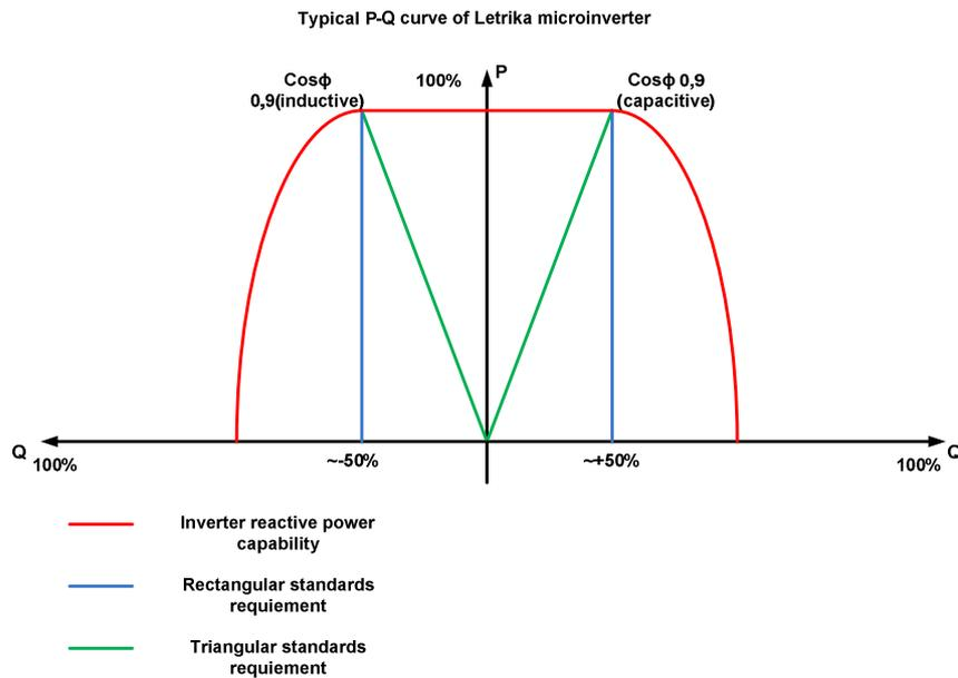
Red line describes inverter reactive power capability. It can be deduced that the inverter can keep real power at nominal level down/up to power factor of 0.9, than the real power will be decreased.
