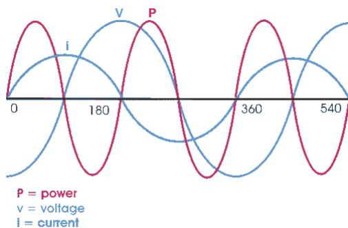
Purely capacitive power. Now the voltage is lagging behind the current. As for inductive reactive power, also here, the useful power is 0.
