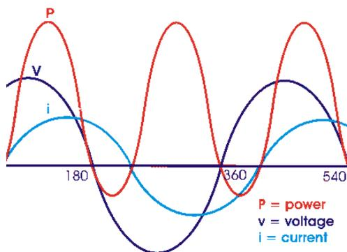
Between two extremes, any combination between real and reactive power is possible. The amount of reactive power is changed with angle between voltage and current.
