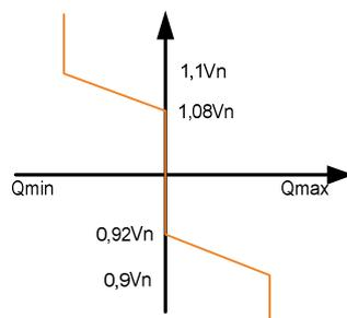
Power factor is linearly changed from minimum to maximum when grid voltage reaches predefined levels.
